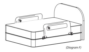
**Step 1:** With the bed rail side in the 'up' position, locate the locking tab on each of the hinges. (*Diagram F*) A close up view of the hinge is shown in (*Diagram G1*).
